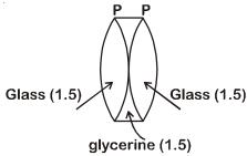
Equivalent focal length in air  $\frac{1}{F_a} = \frac{1}{f} + \frac{1}{f} = \frac{2}{f}$
